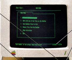
Real-time clock displays time and date on AppleWorks™ screens and files, and is PRO-DOS compatible for use with other PRO-DOS software.
