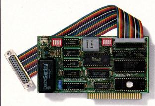
**Serial Pro** is a powerful multifunction card for the Apple IIe, II+, IIGs and compatible computers. Serial Pro combines a powerful serial port for interfacing to a printer, modem or other serial device, with a full function clock/calendar. Serial Pro's serial port is compatible with virtually all letter quality and dot matrix printers, including Apple's Imagewriter and Imagewriter II, and can communicate with the fastest external modems at baud rates from 50 to 19,200.
